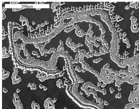
Figure 7. The small-angle grain boundaries and the nearby net-shaped Te-rich phases (the heating rate is 140^\circ\text{C h}^{-1} , and the annealing time is 40 h).
